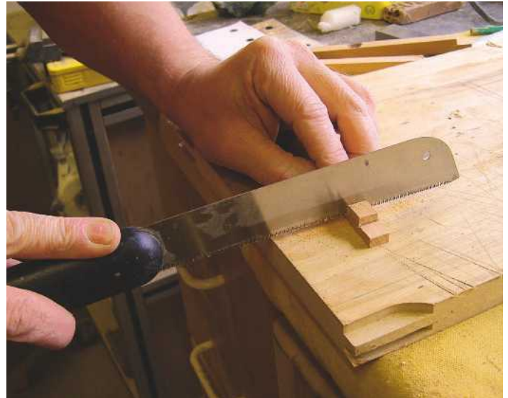
▲ Pic.14 Having cut the step, part the button from the stock. Then drill a countersunk screw hole through
